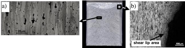
Fig. 4. Structure of the grain on the fracture surface of the AW7075-T7 compact specimen: in the middle of the flat fracture with the rolling direction indicated (a), the edge-side area with plastic strain on the shear lip (b)
