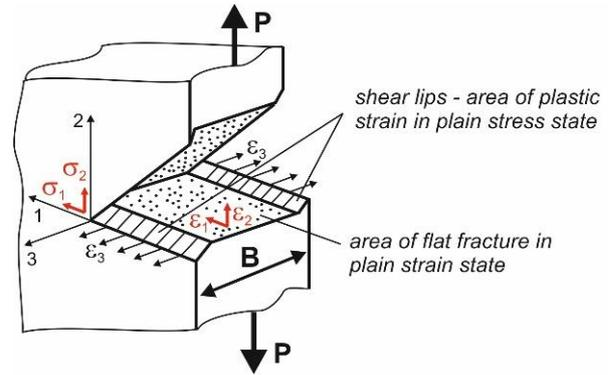
Fig. 2. Systems of strain and stress states on the fracture surface [23]
