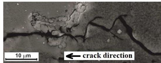
Fig. 7. Fatigue crack arrest mechanism by a second phase intermetallic precipitate in AW7075 material [17]
