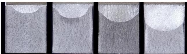
Fig. 5. Propagation of cracks in the AW-7075 material: cracks stopped by shear lips in the RRA, T73, and HTPP aging treatment
