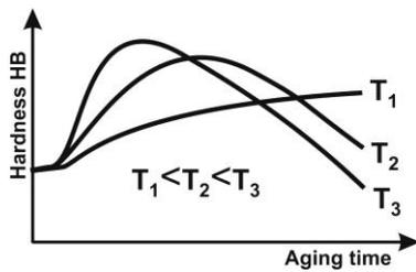
Fig. 1. The influence of temperature and aging time on the hardness of the Al-Cu alloy [12]
