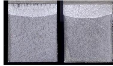
Fig. 6. Flat cracking in the T651 treatment, where the influence of shear lips is much less visible
